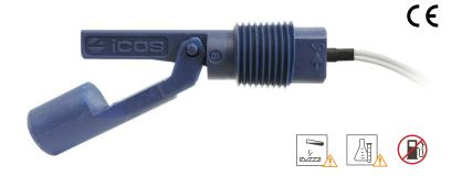
**How it works** Movement of the magnetic float opens/closes a hermetically sealed contact (reed switch).
